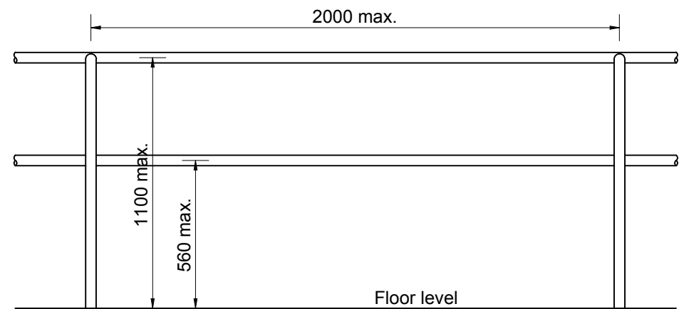
12 Typical Guardrail Detail 1:20
