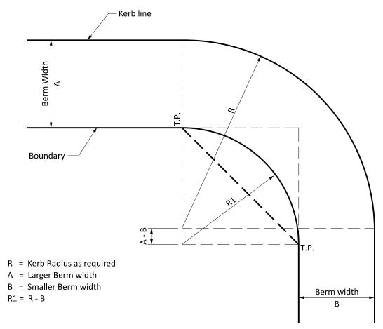
R1 shall be 2000mm Min. and when between 2000mm & 5000mm the boundary shall be a straight line between T.P.'s
