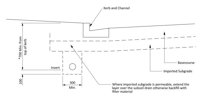
\* Where possible subsoil drainage should desirably be 1000 from top of kerb with suitable outlet to catchpit or manhole
